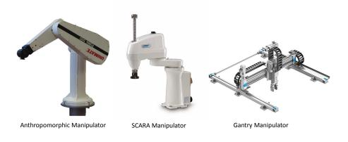
Figure 1: Serial robot examples (anthropomorphic [23], SCARA [14], gantry [22])
