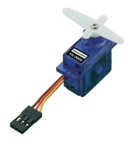
Figure 22: Servo motor [6]
